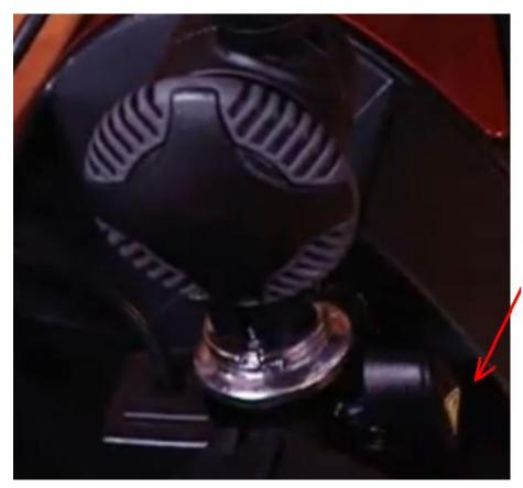
Make sure the steering tiller is turned straight ahead, then push the tiller lock knob in and turn 90 degrees to lock the steering tiller.
