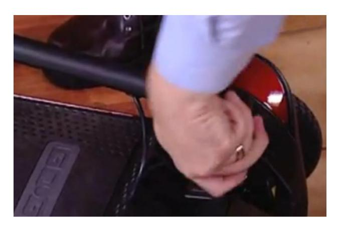
Now raise the steering tiller by loosening the tiller adjustment knob, raising the tiller then retighten.
