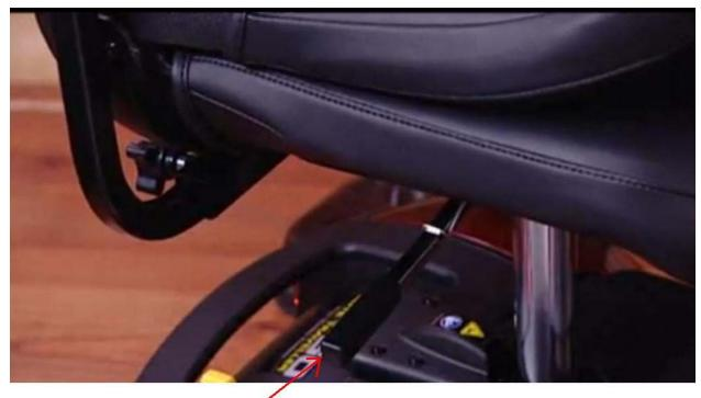
Lift up on the seat release lever and turn the seat and lift to remove the seat
