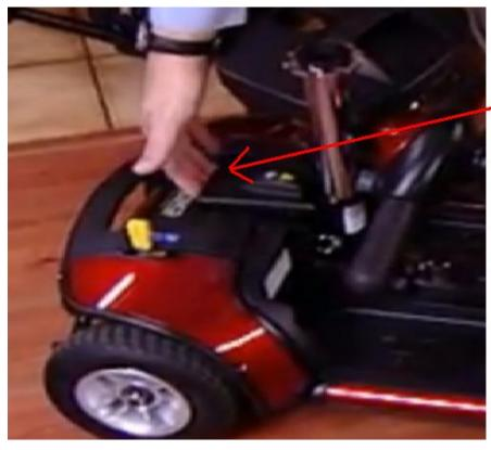
Lift up on the frame release lever
