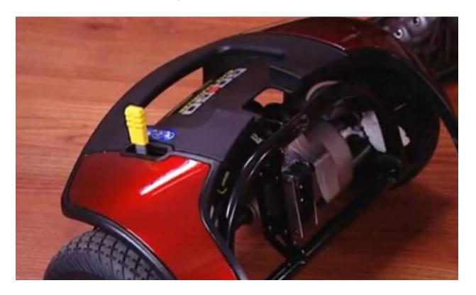
Tip the back part slightly back onto the anti tip wheels
