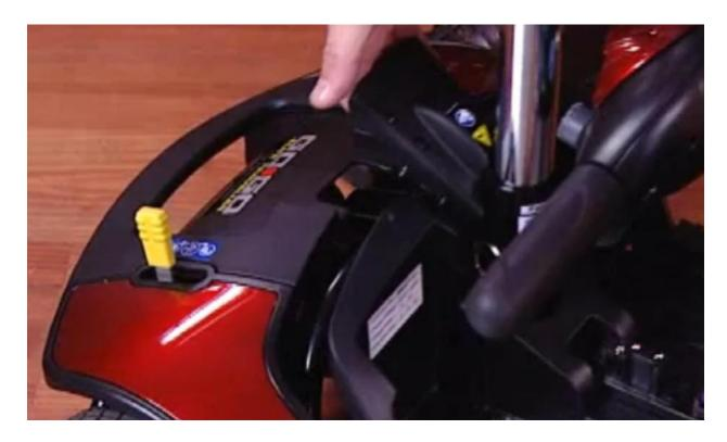
Lift up until the frame hooks are no longer resting on the lower frame tubes
