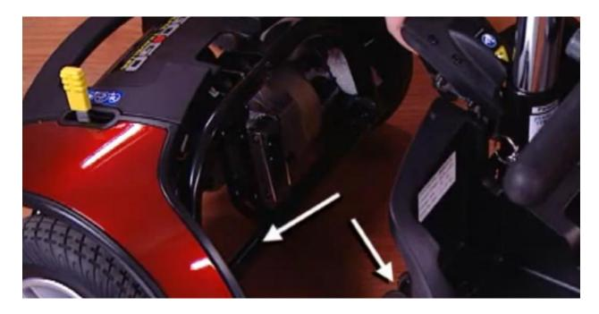
Lift on the frame release level and align the hooks on the front section over the frame tube of the rear section.
